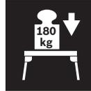
The maximum load bearing capacity (power tool + workpiece) of the saw stand is **180 kg**.
