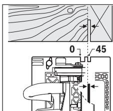
The 0° cut mark (8) indicates the position of the saw blade when making a right-angled cut. The 45° cut mark (9) indicates the position of the saw blade when making a 45° cut. For a precise cut, place the circular saw against the work-piece as shown in the figure. We recommend making a test cut.
