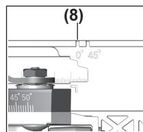
Use only cut marks (8) when making a right-angled cut and a 45° cut with the guide rail.
