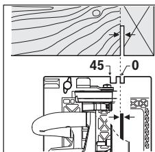
The 0° cut mark (9) indicates the position of the saw blade when making a right-angled cut. The 45° cut mark (8) indicates the position of the saw blade when making a 45° cut. For a precise cut, place the circular saw against the work-piece as shown in the figure. We recommend making a test cut.
